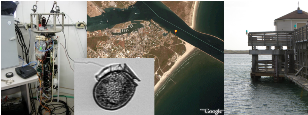
Imaging Flow Cytobot in the lab of Dr. Lisa Campbell (Texas A&M University) identified HAB cells from water sampled at the Port Aransas Pier. (Photos: Campbell)
