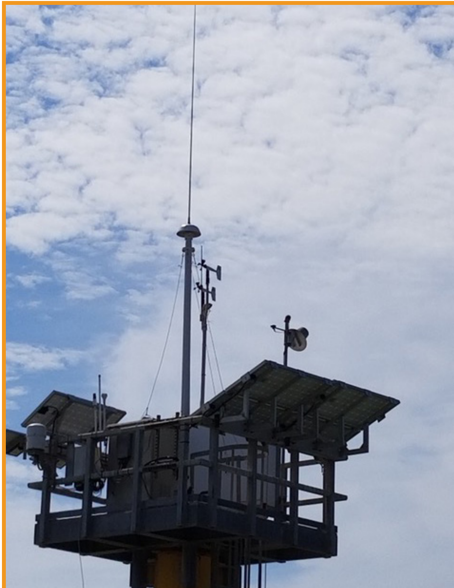
Figure 4. This single antenna long-range SeaSonde is an HFR alternative for some locations.
