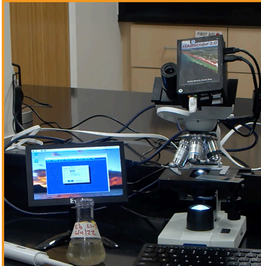
Figure 7. HABscope 2.0 utilizes a Raspberry Pi computer to process and upload video to the cloud.
